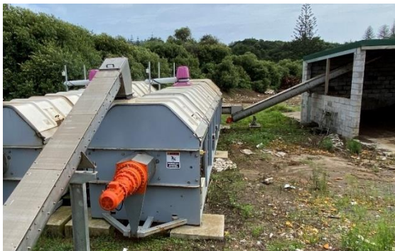
Image 6: HotRot and BiobiN in-vessel systems
